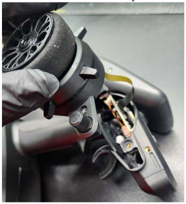
Carefully lift the black lever on the radio side to release the ribbon cable.
