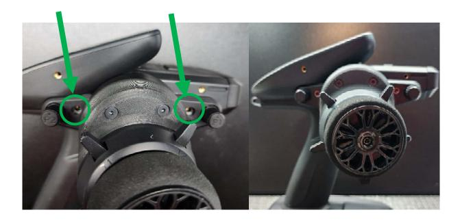
These two black Phillips screws are NOT used in with the VSR Products drop down kit.
